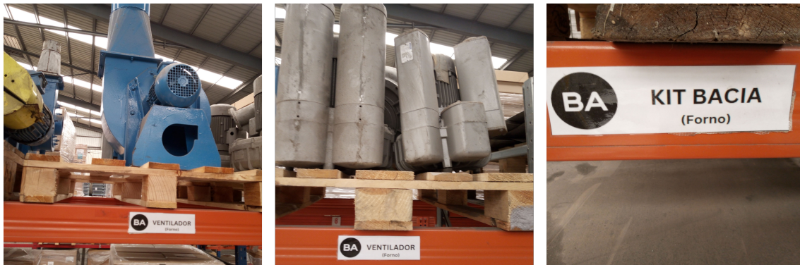
Figure 4.9: Provisional spare part identification
