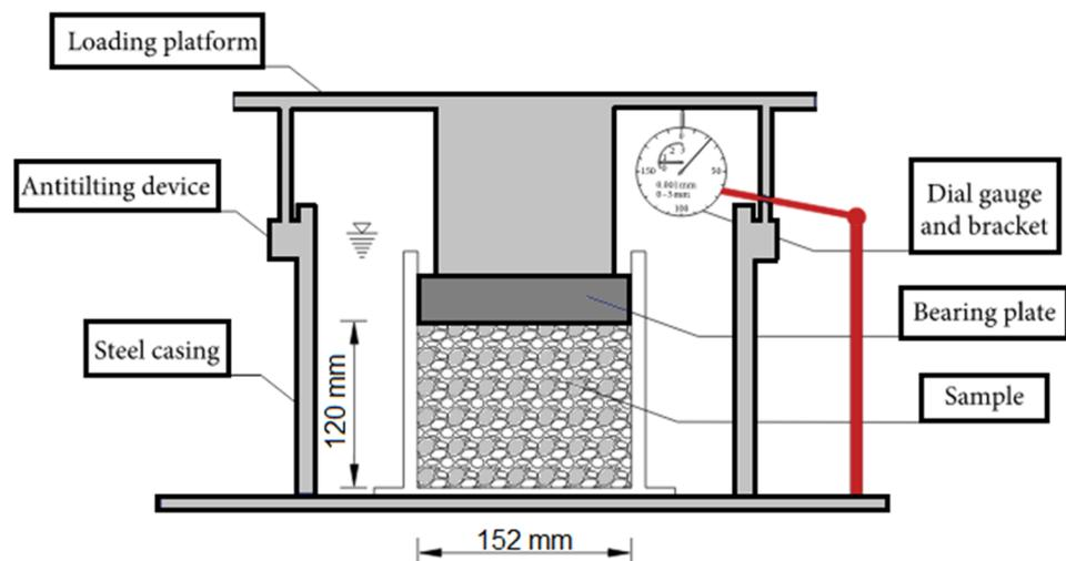
Figure 10. Creep loading tests apparatus used by Li et al. (adapted from [117]).
