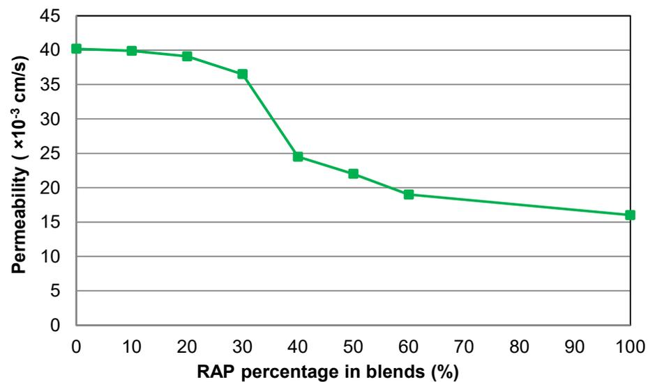
**Figure 6.** The permeability test results of RAP/natural aggregate blends [108].
