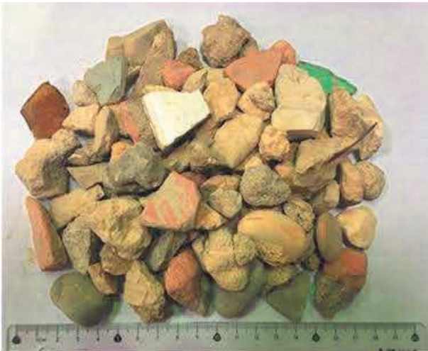
Figure 1. Sample of the recycled aggregate used (ruler in centimetres).
