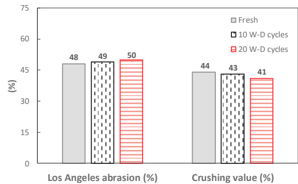
Figure 9. Effects of W-D cycles on resistance to fragmentation and crushing.
