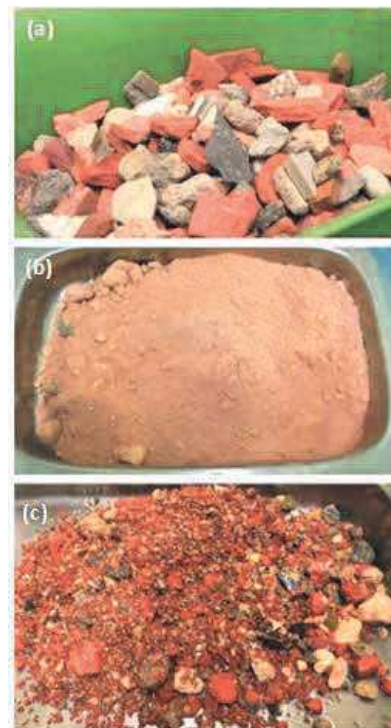
Figure 10. Fresh sample appearance in LA abrasion test: (a) before going into the testing machine; (b) after getting off the testing machine; (c) after washing.
