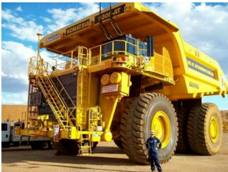
Figure 3 - Anglo American ultra-heavy-duty mining truck to be retrofitted with 800kW of fuel cell modules [11]
