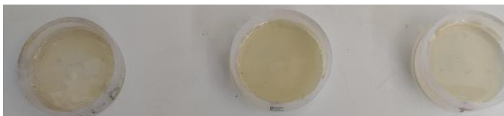
Figure 13 - Film of the binder or crosslinker/binder system on teflon circular plaques.
