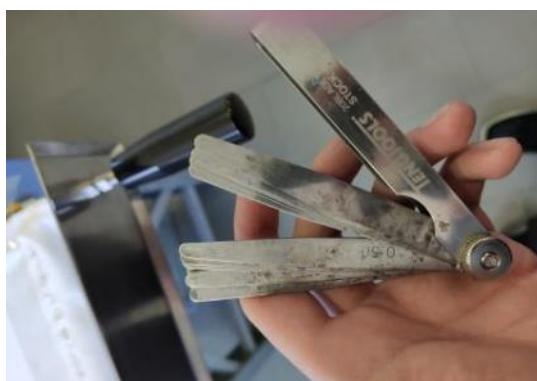
Figure AP-2 - Feeler gauge set employed to measure coating thickness.
