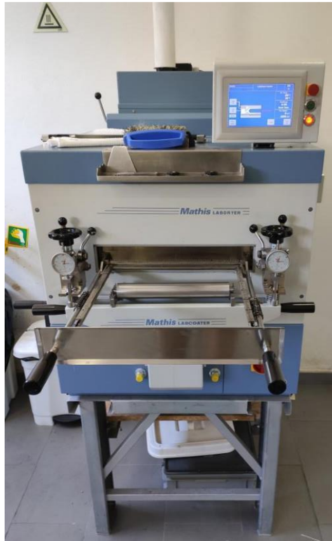
Figure AP-3 - Mathis Labcoater type LTE-S.
