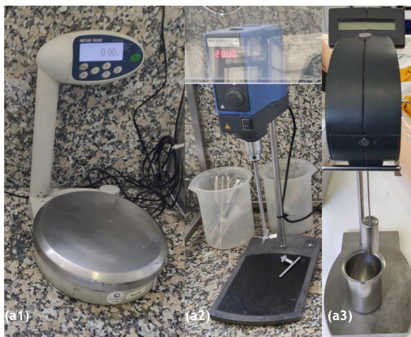
Figure AP-1 - (a1) Scale used to weight the coating ingredients, (a2) stirrer utilized to mix them, and (a3) viscotester employed to measure the viscosity of the blend.
