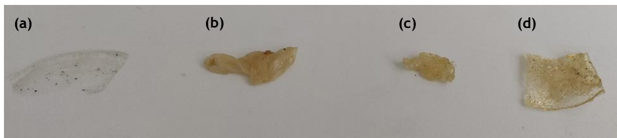
Figure E-1 - Mixture of Impranil DLN-SD with (a) Imprafix 2794, (b) Acrafix EP 6047, (c) Arkophob DAN New liq at a 33/67 mass ratio. (d) Impranil DLN-SD by itself.
