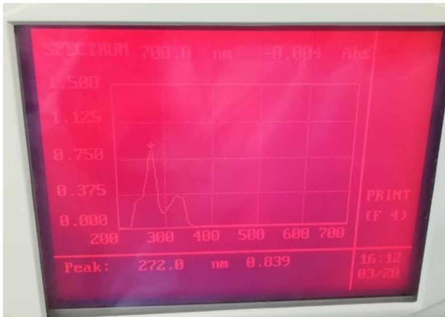
Figure II.2 - Emission spectrum of a ciprofloxacin sample with a concentration of 10.00 \times 10^3 \mu\text{g L}^{-1} .
