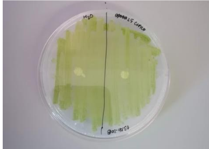
Figure XIII.1 – Paper-disc agar method with a ciprofloxacin concentration of 2.50 \times 10^3 \mu\text{g L}^{-1} and water as blank.
