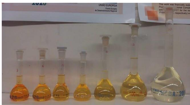
**Figure 2** – Solutions prepared for the calibration line for  $\text{H}_2\text{O}_2$  measurement.
