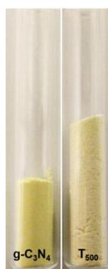
**Figure 9** – The same amount (50 mg) of *bulk* g-C<sub>3</sub>N<sub>4</sub> and after thermal post-treatment (T500).
