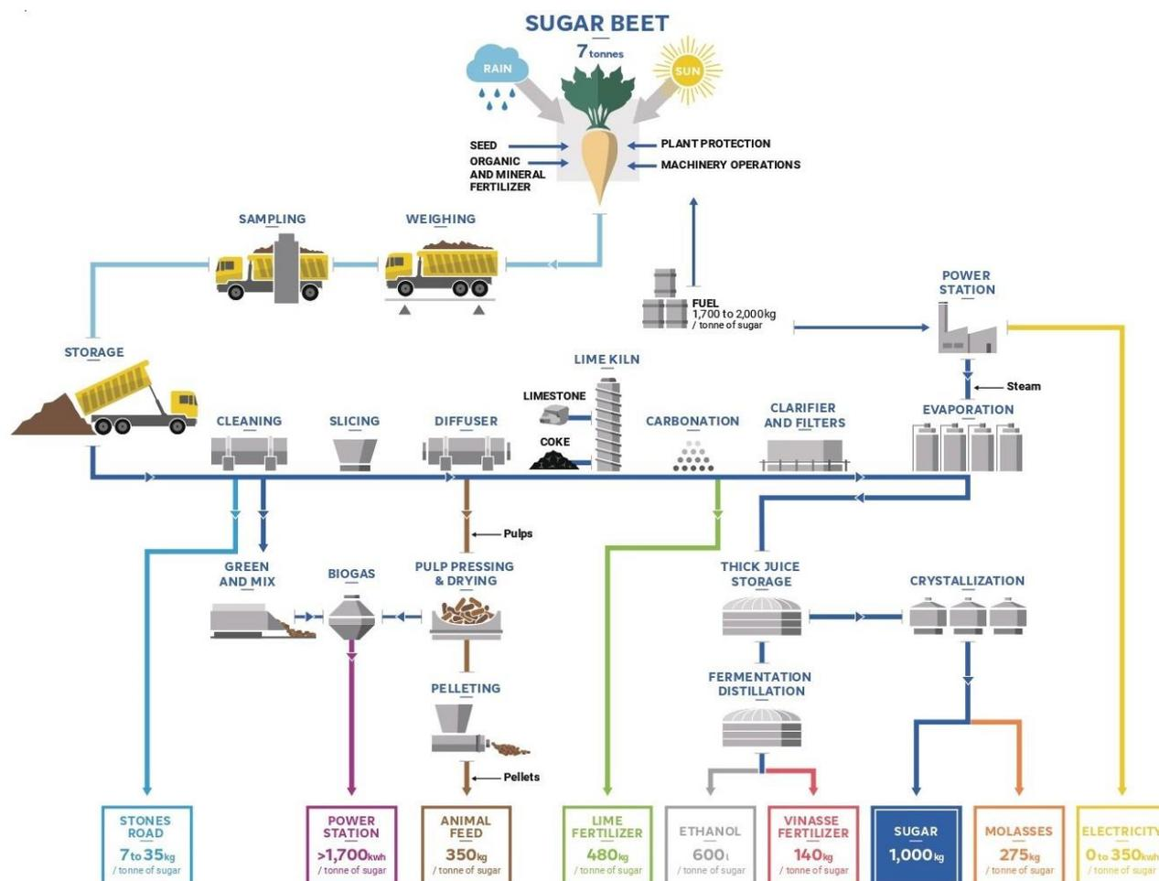
Figure 2 - Sugar beet processing from harvesting to formation of sugar and by-products (Sucden, 2020).
