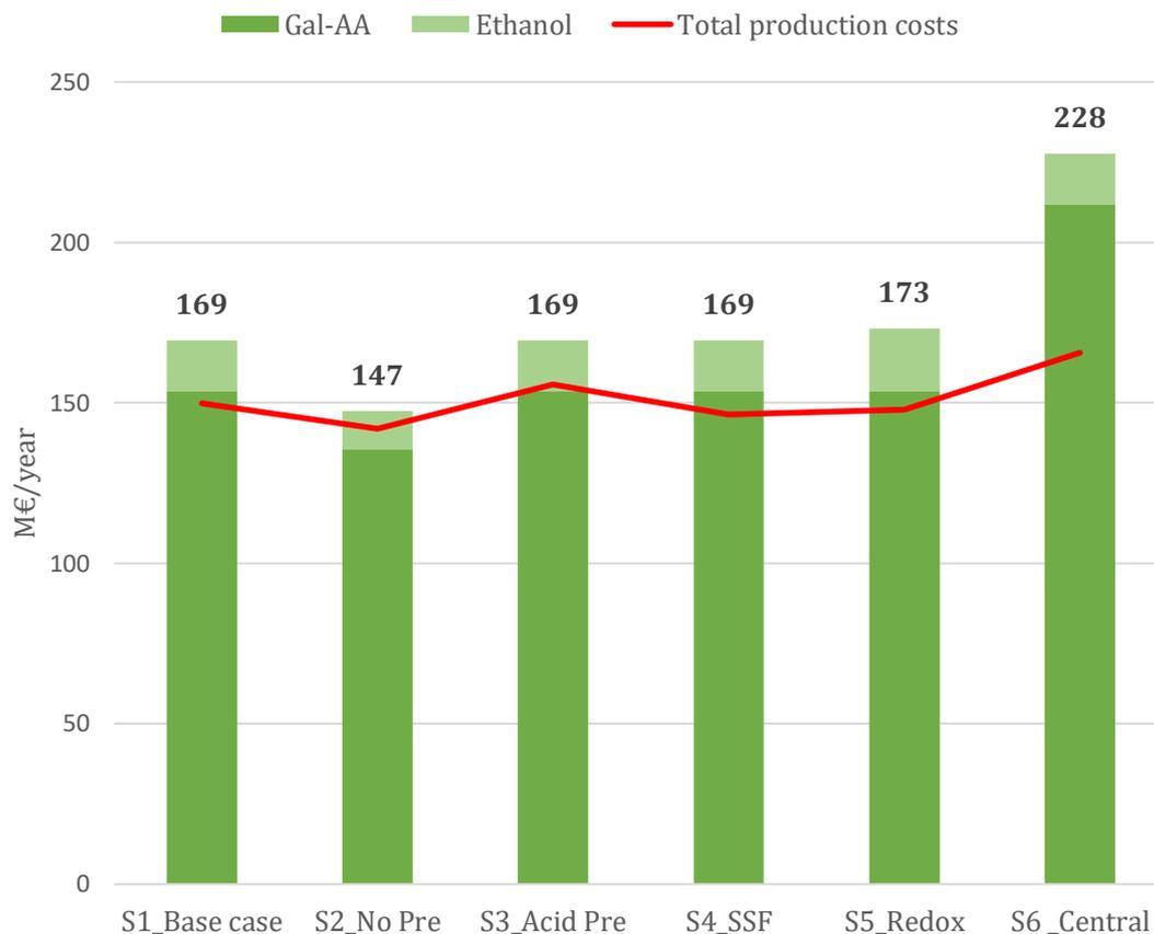
Figure 20 – Total revenues of products sold (separated per product) and total production costs for all studied scenarios. Gross margin is graphically represented through the distance between the top of the bar and the red line.
