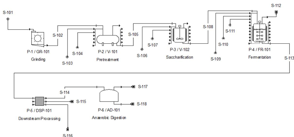
Figure 17 – Process diagram for the envisioned galactaric acid production.
