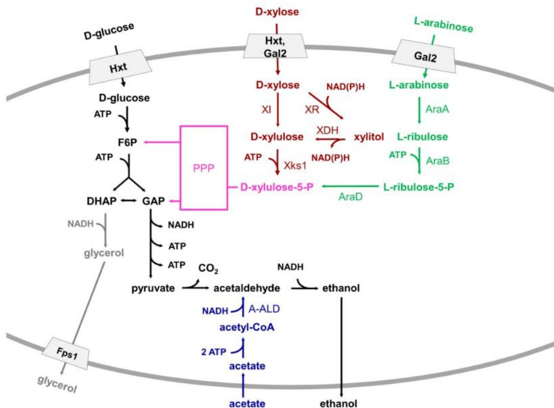
Figure A1 - Key strategies for engineering carbon and redox metabolism in *S. cerevisiae* strains for alcoholic fermentation of lignocellulosic feedstocks (Jansen *et al.*, 2017).
