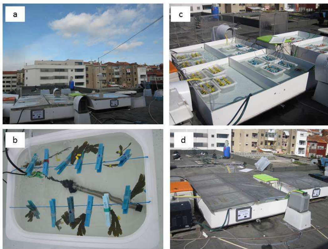
Figure 4. a) General view of the outdoor seawater tanks system used for the seawater stress experiments, b) Detailed view of each chamber, containing the titanium heater and the temperature probes, c) Seawater 20 l tanks submersed in the water bath system, d) General view of the outdoor system covered with the fiberglass mesh, reducing 33% of the incident light.
