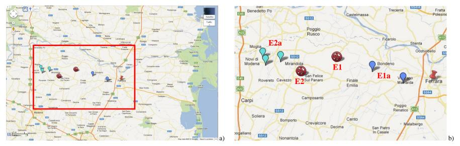
Fig. 1 – Location of the epicentres of the main events of the Emilia-Romagna earthquake sequence: general overview (a); detailed view (b): E1) earthquake of the  $20^{th}$  May, E1a) aftershocks of the  $20^{th}$  May earthquake with magnitude  $M_w > 5.0$ , E2) earthquake of the  $29^{th}$  May, E2a) aftershocks of the  $29^{th}$  May earthquake with magnitude  $M_w > 5.0$ .
