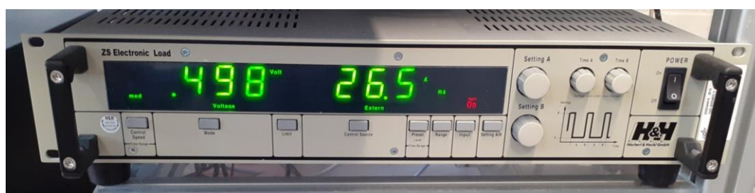
Figure 6 external ZS electronic load used on potentiostic mode
