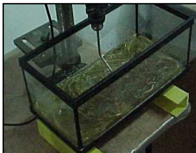
Figure 3: Sodium Hydroxide bath
