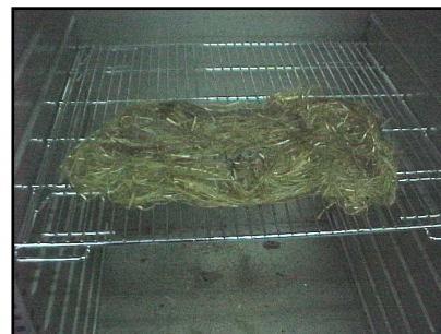
Figure 4: Fibres in the oven
