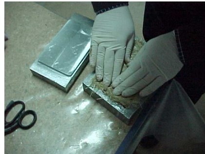
Figure 7: Placing the mat
