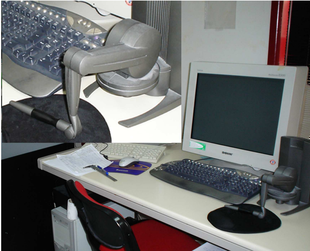
Figure 3 - Haptic device for virtual sculpting (Phantom Omni).
