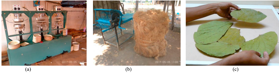
Fig. 3. a) Pressed Areca plates; b) Coconut fiber ready for being processed; c) Sal leaves being stitched.
