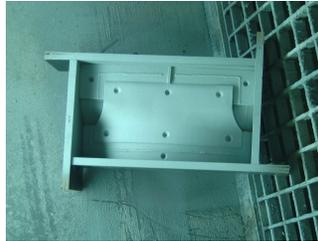
Fig. 6 - Half mould after deposition of the metallic coating.
