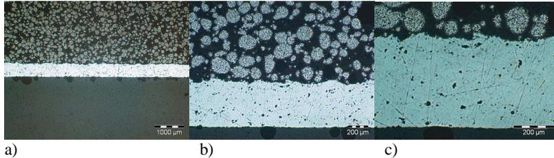
Fig. 8 - Cross-section of one mould composed by a metallic layer and a back up in composite resin; a) cross section of the mould; b) detail of the two phases; c) detail of the metallic shell, showing small round black dots, corresponding to the shell porosity.
