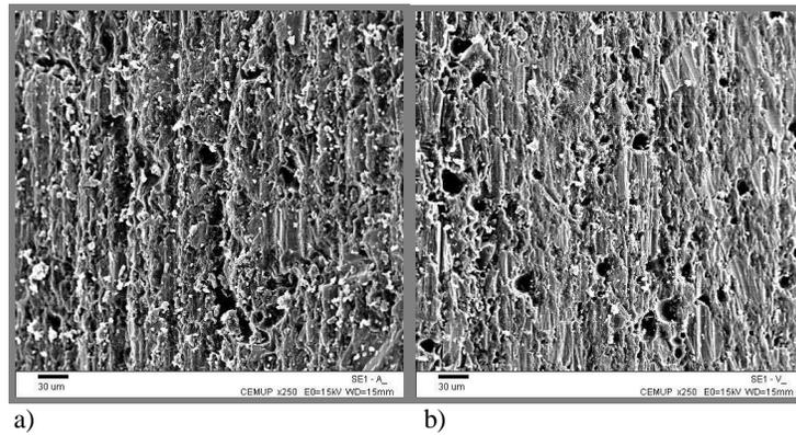
Fig. 15 - SEM images of the moulding cavity surfaces, revealing the degree of excoriation occurred in the thermoplastic flow direction of the: a) AF mould with more severe excoriation, deeper grooves, and; b) AFG moulds, with softer surfaces.
