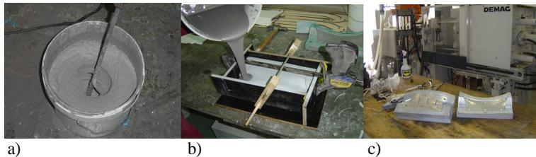
Fig. 7 - Back up of the first half mould: a) mixing of the resin with the catalyst and the aluminium metallic particles; b) casting the slurry over the metallic shell; c) final mould.
