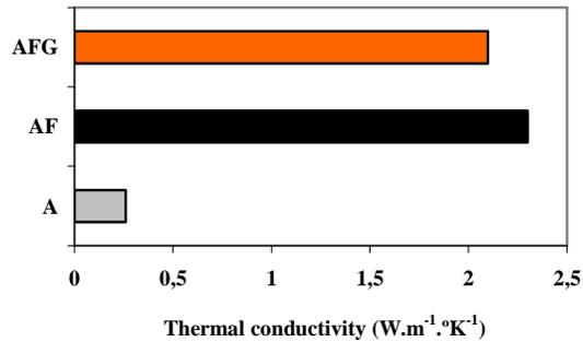
Fig. 12 - Thermal conductivity of the three tested materials (Kirksite alloy Z35541 – ASTM B86 [14] has 105.0 W.m<sup>-1</sup>.°K<sup>-1</sup>).
