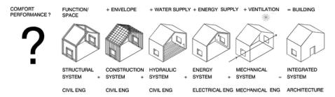
Fig. 3. Integrated Design Concept [21].
