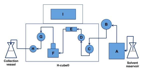
Figure 35. H-cube® scheme. A - pump; B - Manual injector; C - inlet pressure sensor; D - gas-liquid mixing chamber; E - bubble detector; F - CarCart® holder and heating unit; G - outlet pressure sensor; H - back pressure regulator; I - touch screen panel. Arrows indicate the flow direction. Adapted from (Bryan, Wernick, Hein, Petersen, Eschelbach, & Doherty, 2011)
