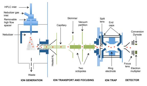
Figure 41. Trap mass spectrometer for ion transmission and detection
