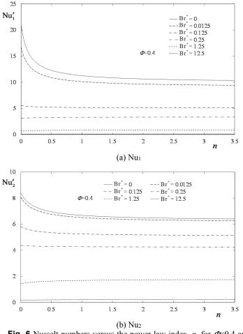
**Fig. 6** Nusselt numbers versus the power-law index, n, for  $\Phi$ =0.4 and different values of the Brinkman number, Br<sup>\*</sup>. Data obtained using two bulk temperatures, the new approach.
