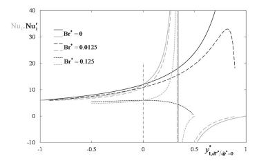
Fig. 9 Nusselt number, Nu₁, versus the corresponding coordinate of the location of the temperature profile where ∂*T*/∂*y*=0, y<sup>\*</sup><sub>1,dT</sub>\*/y<sup>\*</sup>=0</sub>, for different values of the Brinkman number, Br\*, and *n*=0. Lines: Grey lines – "classical" approach, black lines - new approach, the vertical line marks the duct axis coordinate..
