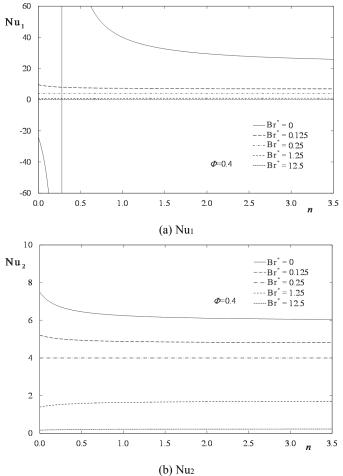
**Fig. 3** Nusselt numbers versus the power-law index, n, for  $\Phi$ =0.4 and different values of the Brinkman number, Br\*. Data obtained using the "classical" approach for the bulk temperature calculation.
