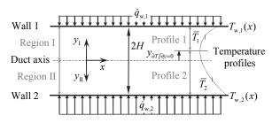
Fig. 1 Schematic representation of the parallel plates duct, the boundary conditions and of the coordinate systems. A temperature profile is also shown, which is divided by the point where  $\partial T/\partial y=0$ .
