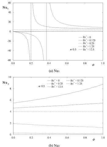
**Fig. 4** Nusselt numbers versus the wall heat flux ratio,  $\boldsymbol{\Phi}$ , for n=0.5 and different values of the Brinkman number, Br\*. Data obtained using the "classical" approach for the bulk temperature calculation.
