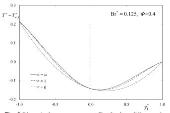
**Fig. 2** Dimensionless temperature profiles for three different values of n, Br<sup>\*</sup>=0.125 and  $\Phi$ =0.4. The vertical line represents the duct axis.
