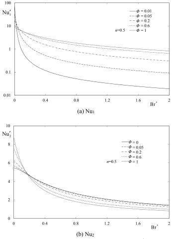
Fig. 8 Nusselt numbers versus the Brinkman number, Br\*, for n=0.5 and different values of the wall heat flux ratio, Φ. Data obtained using two bulk temperatures, the new approach.
