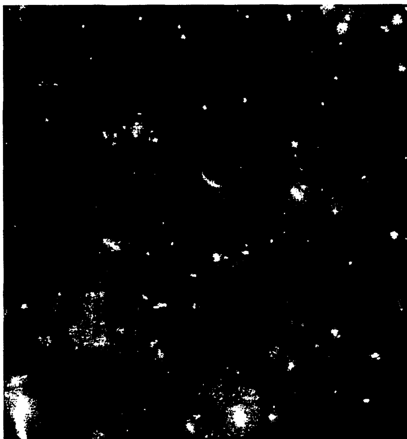
FIGURE 6 Epifluorescence micrograph of a stainless steel coupon after exposure for 1 h to a bacterial suspension treated with 300 \text{ mg l}^{-1} of biocide. \times 400 (See Colour Section.)
