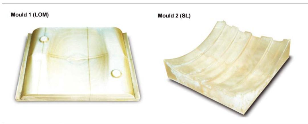
Fig. 3. LOM and SL moulds after finishing operations.
