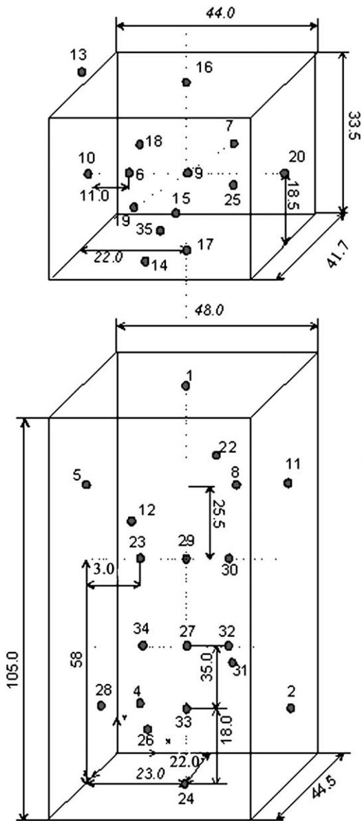
Fig. 2. Location of the thermocouples inside the refrigerator-freezer.
