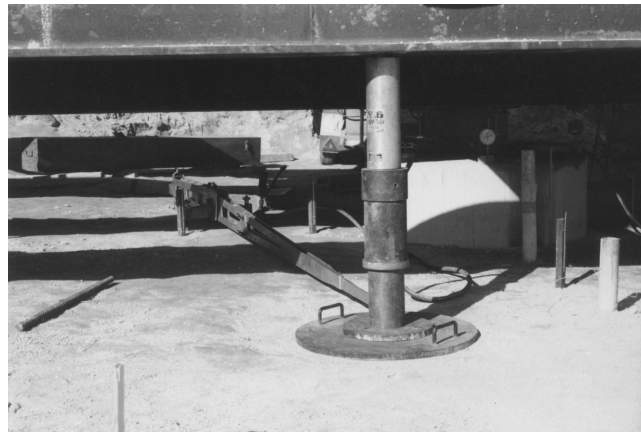
Figure 18. Plate loading test (D = 60 cm).
