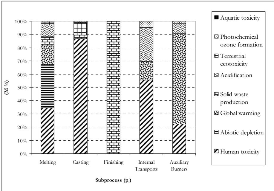
Figure 4.4. The relative contribution of sub-process ( $p_i$ ) to different environmental problems (using the valuation method that considers all problems equally important), and assuming no implementation of reduction options (unit: % relative to the M).
