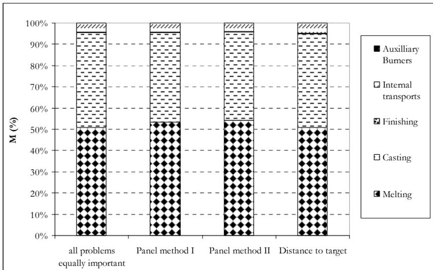
Figure 4.3. The contribution (%) of each sub-process of an aluminium die casting plant to the overall environmental impact ( $M$ ) for four Multi-Criteria Analysis (MCA) approaches taking different valuation methods: All problems equally important, Panel Method I (Kamp, 2005), Panel Method II (Kortman et al., 1994), Distance to target (Goedkoop, 1995). (unit: % relative to the  $M$ ).
