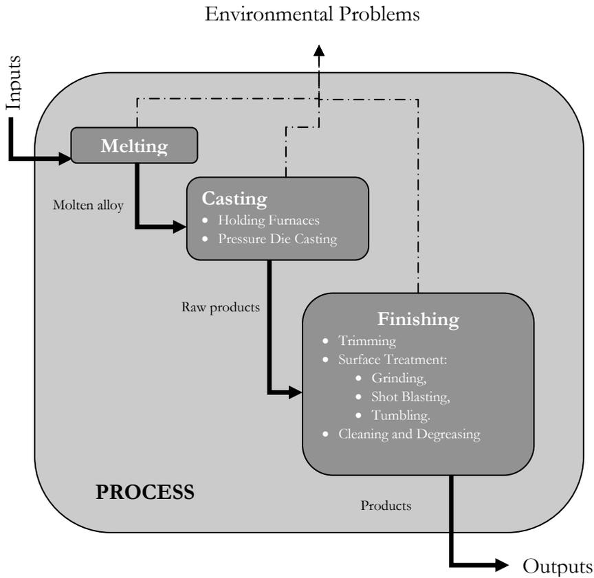
Figure 4.1. The aluminium pressure die casting plant's production line. The figure includes the sub-processes and sub-sub-processes that we included in our model (see also Table 4.1). The scheme includes the alloy mass flow throughout the production line. Part of the alloy mass flows exiting Casting and Finishing are recycled internally. For simplification, these flows of recycled alloy are excluded from the figure.
