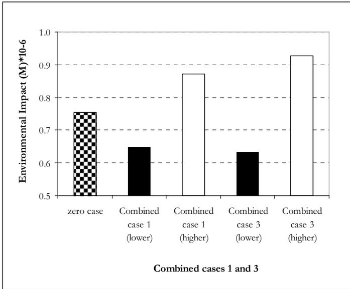
Figure 4.5. The calculated overall environmental impact (M) for two combined cases, in each of which was changed the value of a parameter to a lower or higher value, in order to test the sensitivity of the model results to changes in parameter values. The *zero case* uses parameter values as presented in earlier sections of this chapter. The valuation method used considers all environmental problems to be equally important.
