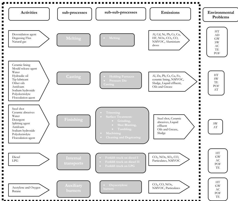
Figure 3.1. Overview of an aluminium die casting plant including activities (inputs of energy and subsidiary materials) into the (sub-)sub-processes, emissions of pollutants and the associated environmental problems. The dotted line indicates the system boundary (gate-to-gate). HT= Human Toxicity; AD= Abiotic Depletion; GW = Global Warming; SW = Solid Waste production; AC = Acidification; TE = Terrestrial Ecotoxicity ; POF = Photochemical Ozone Formation; AT = Aquatic Toxicity.
