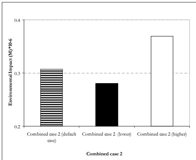
Figure 4.6. The calculated overall environmental impact (M) for Combined case 2, in each of which the value of a parameter was changed to a lower or higher value, in order to test the sensitivity of the model results to changes in parameter values. The calculation of M for *Combined case 2* (default case) uses the default parameters for the situation when the reduction options were implemented. The valuation method used considers all environmental problems to be equally important.
