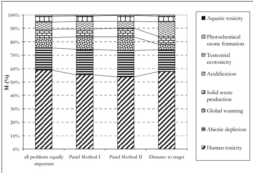
Figure 5.1. The relative contribution (%) of environmental impact categories ( $z$ ) to the overall environmental impact ( $M$ ) of an aluminium die casting plant for the zero case. Results are shown for four multi-criteria analyses (MCA) using different valuation methods: All problems equally important; Panel Method I (Kamp, 2005); Panel Method II (Kortman et al., 1994); and Distance to target (Goedkoop, 1995). (units: % relative to  $M$ ).
