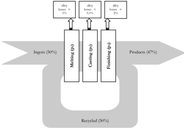
Figure 4.2. Alloy mass flow on the existing aluminium pressure die casting plant.
