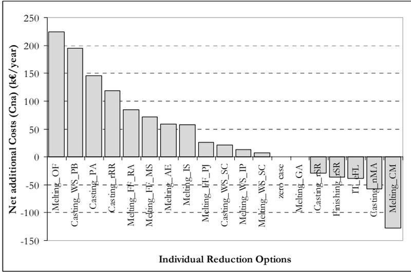
Figure 5.5. Net additional Costs ( $C_{na}$ ) for the aluminium die casting plant for cases in which it is assumed that one of the reduction options is implemented. See Table 5.2 for an explanation of reduction options.
