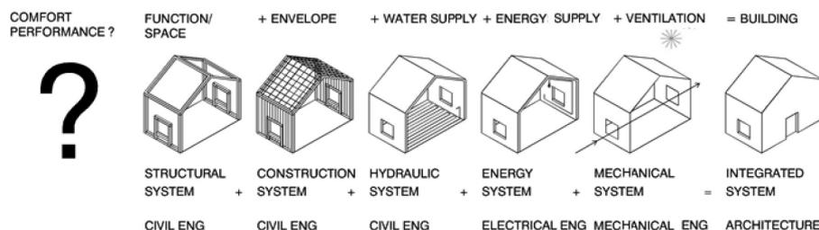
Fig. 3. Integrated Design Concept [21].
