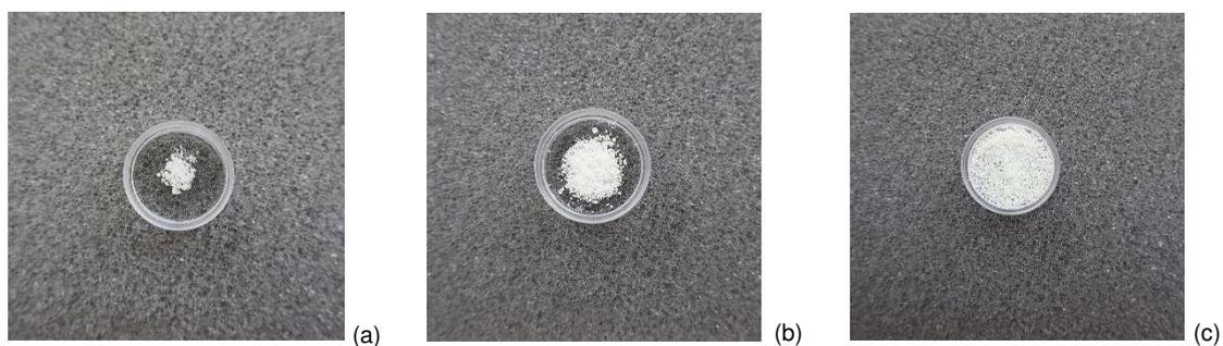
Figure 3.24. Typical amounts of sample used for the solid state fluorescence measurements (approximate percentage of the area of the base of the dish covered by powder sample: a. 15 %; b. 40 %, c. 100 %).
