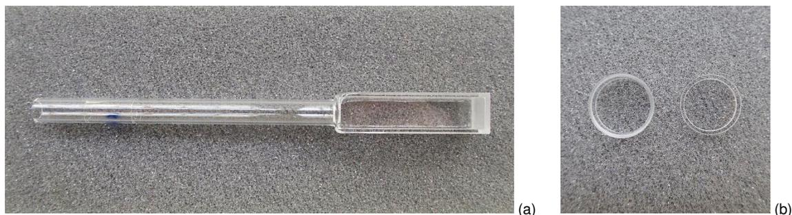
Figure 3.23. Quartz cuvette (a) and lidded petri dish (b) used for the fluorescence measurements in solution and in the solid state, respectively.
