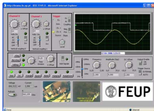
Figure 1. A remote workbench supporting basic electronics experiments
