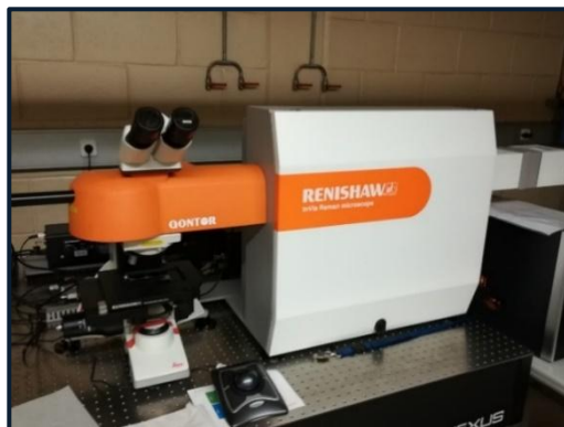
Figure A.6. Experimental setup: Raman spectrometer. System inVia Qontor, Renishaw®.
