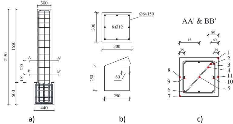
Fig. 1 - Geometry and reinforcement detailing: a) global dimensions; b) cross-section; c) location of thermocouples (dimensions in mm).
