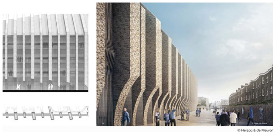
Fig. 7 Detail of the facade—elevation and plan; west elevation and Oswald Stoll Mansions, Herzog de Meuron (2015), Stamford Bridge Grounds. Detailed Plan Application. Design and Access Statement [4, pp. 115 and 140]
