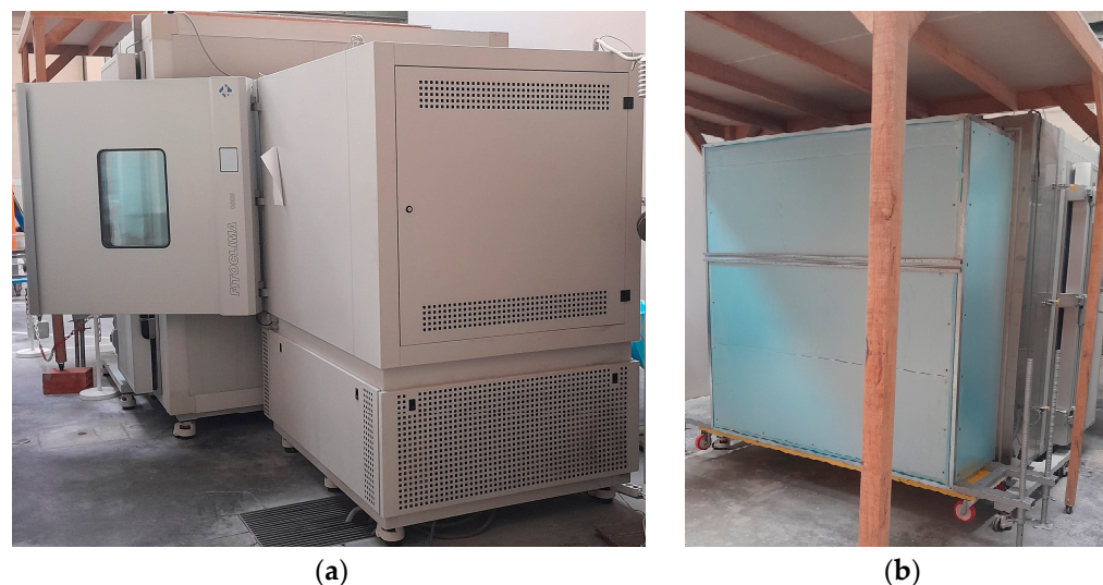
Figure 1. Apparatus for hot box method: (a) hot side; (b) cold side.
