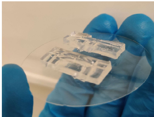
Figure 3.13: Half chips on the disc prepared for the binding process.
