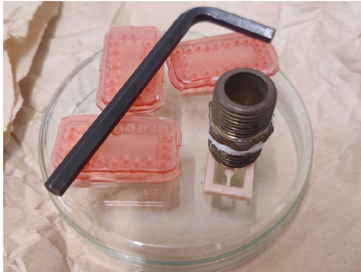
Figure A.10: Mould setup with support material between weights and mould.
