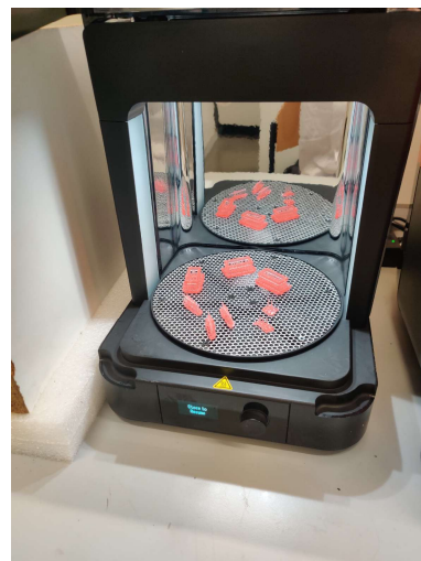
(b) UV treatment in the Formlabs Form Cure machine.
