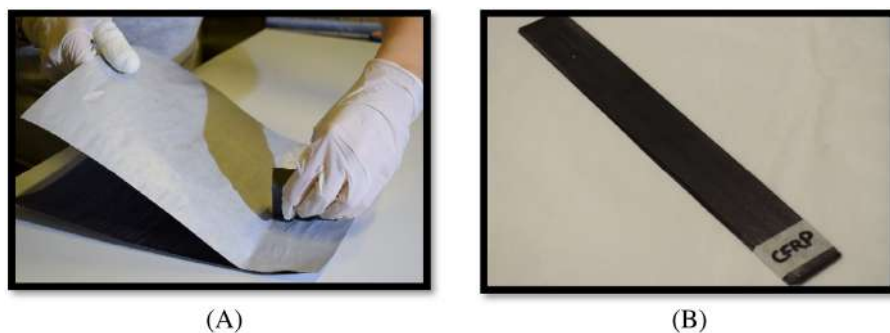
FIGURE 1 (A) Layer-by-layer stacking of the composite prepreg and (B) conventional composite plate
