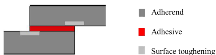
Figure 27. Localised surface toughening concept. Adapted from [161].
