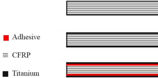
Figure 2.8: Studied configurations by Santos et al. [115] for CML and CMLs with additional adhesive layers.
