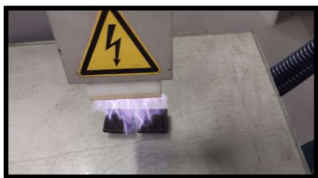
FIGURE 5 Plasma treatment for thin-ply blocks
