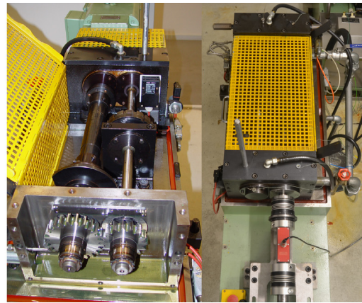
Fig. 2. Schematic view of the FZG gear test rig.
