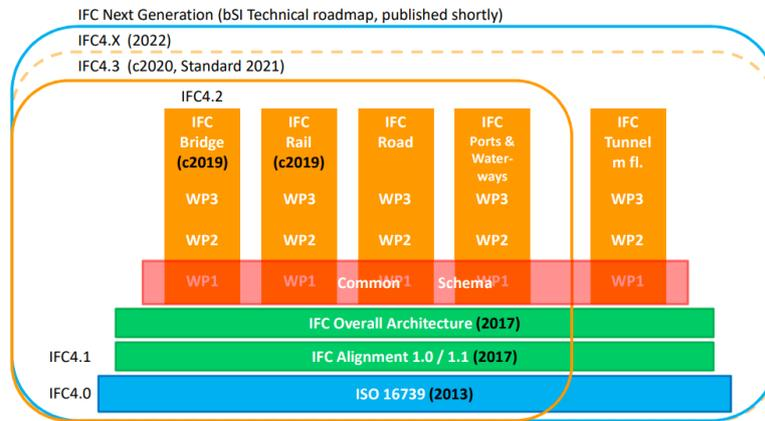
Figure 1 – IFC expansion for horizontal infrastructures (buildingSMART International Ltd. 2022)
