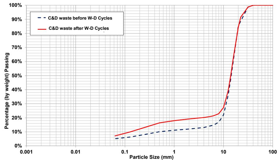
Figure 9. Grain size distribution for recycled C&D aggregate before and after W–D cycles (adapted from [116]).
