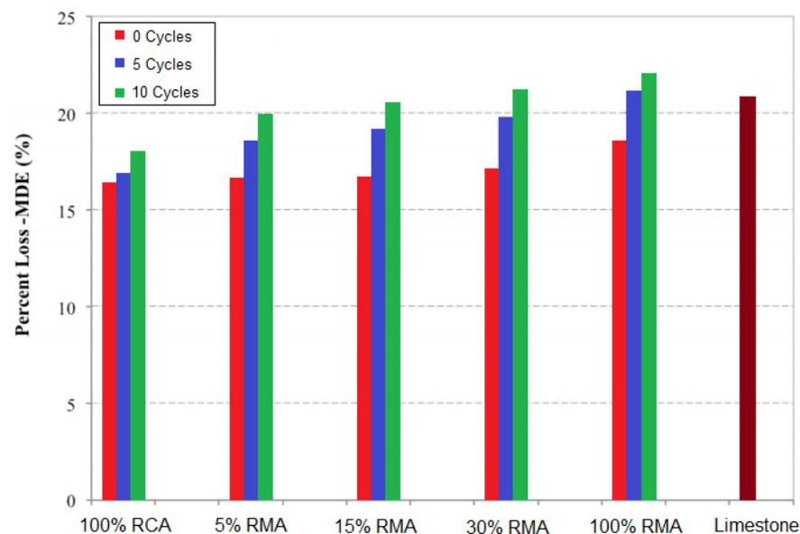
**Figure 8.** Percent loss of the Micro-Deval coefficient of the natural and recycled aggregates submitted to different number of W–D cycles (adapted from [110]).
