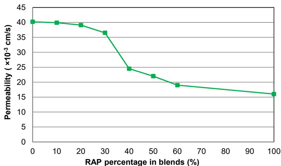
**Figure 6.** The permeability test results of RAP/natural aggregate blends [108].
