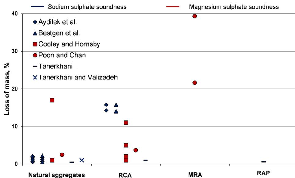
**Figure 7.** Sodium sulphate and magnesium sulphate soundness of natural and recycled aggregates (RCA—recycled concrete aggregate; MRA—mixed recycled aggregate; RAP—reclaimed asphalt pavement) [18,78,89–91,93].
