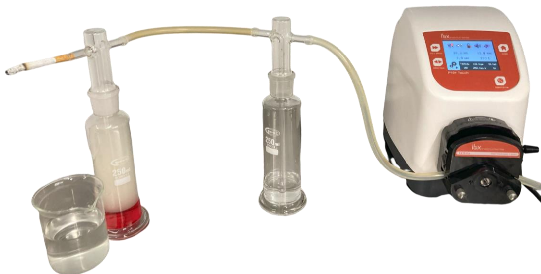
Figure 2 - Experimental set-up: Generation of conventional cigarette smoke
