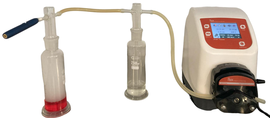
Figure 3 - Experimental set-up: Generation of IQOS 3™ aerosol
