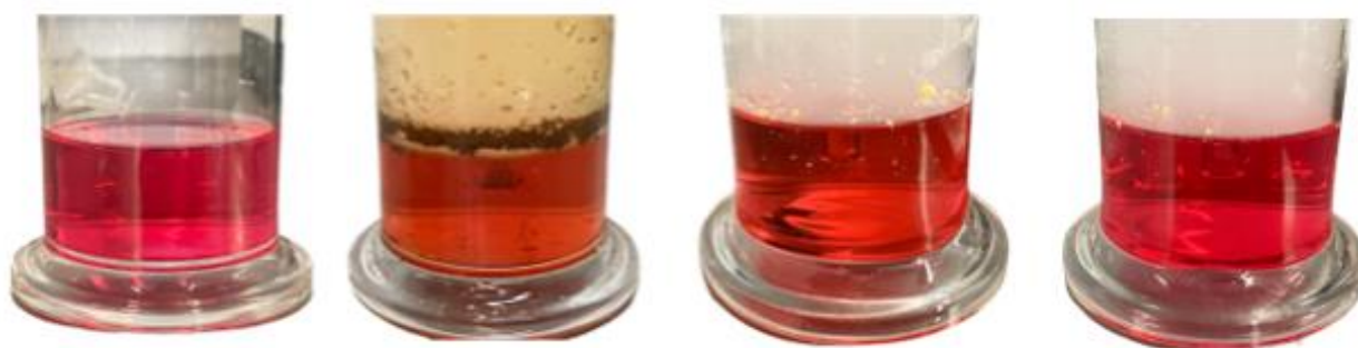
Figure 6 - Deposit matter following different exposures (from left to right: control, CS, IQOS 3™, IQOS ILUMA ONE™)
