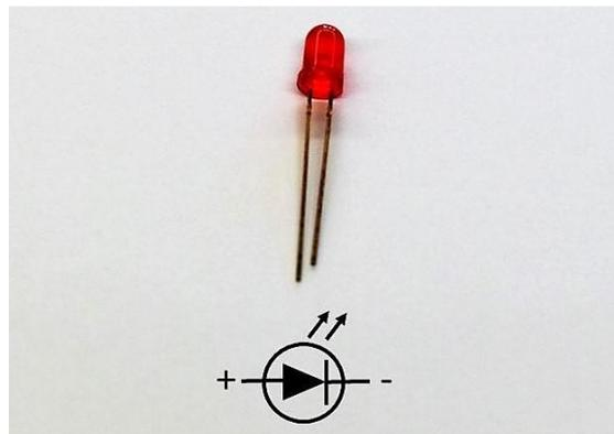
Figure 2: Photograph and schematic representation of a LED. The long leg corresponds to the positive pole. Source: own authorship.
