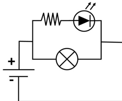
Figure 4: Electric circuit with a 3 V battery and lead wires. A protective resistance of  $220\ \Omega$  is series with the LED is mounted in parallel with a lamp. Source: own authorship.
