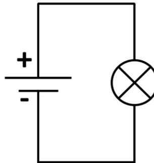
Figure 3: Circuit with a bulb lamp, lead wire and a 3 V battery. Source: own authorship.
