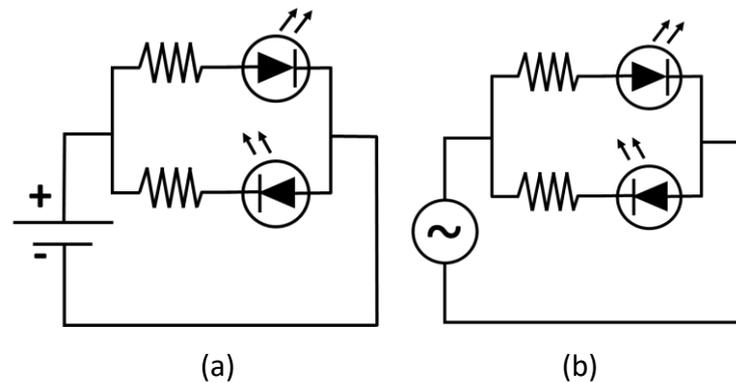
Figure 5: Electric circuit with lead wires, where two LEDs are mounted in parallel with (a) a 3 V battery, and (b) an AC 3 V generator. Each LED has in series a protective resistance of  $220 \Omega$ . Source: own authorship.
