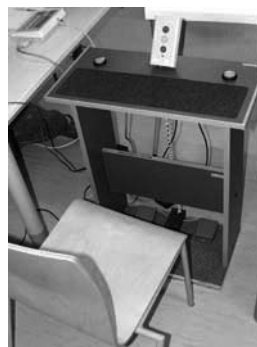
Figure 1 – Reaction time measurement device (MCR 2001E) by Psychotronics. Photograph by the authors.
