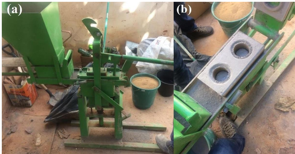
Figure 3. Production equipment: (a) Manual press for manufacturing ecological brick, (b) Ecological brick after pressing.
