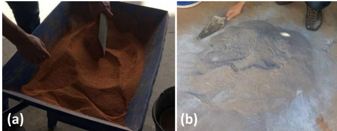
Figure 2. (a) Aggregate of waste ceramic materials passing through the sieve 16, and (b) Mixing raw materials before molding.
