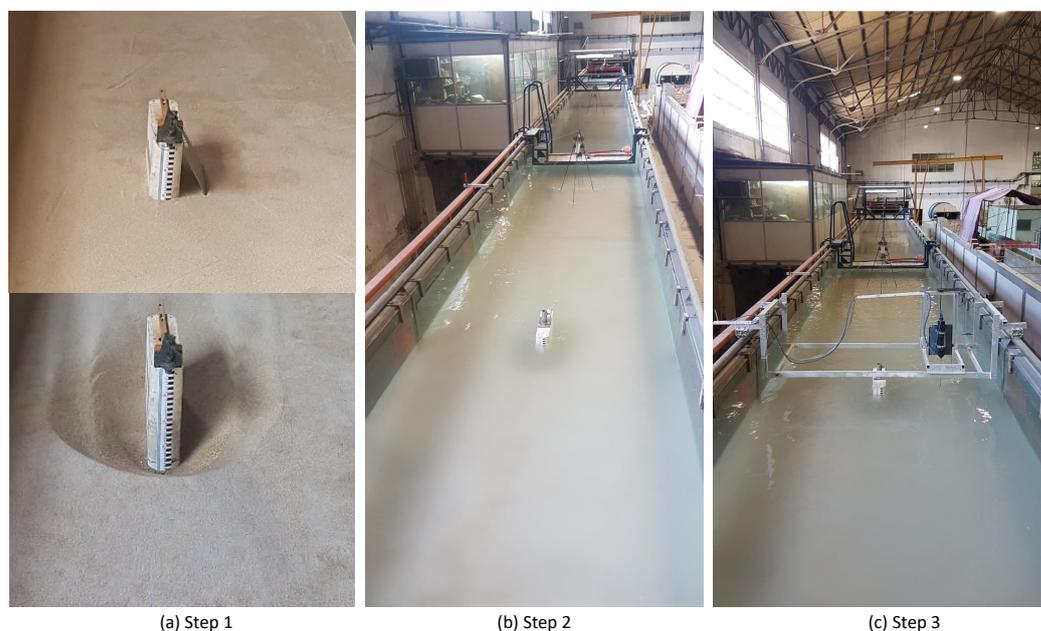
**Figure 4.** Setup for the flow velocity measurements.
