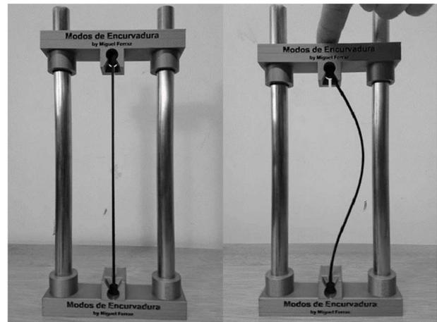
Fig. 8. Using the buckling model
