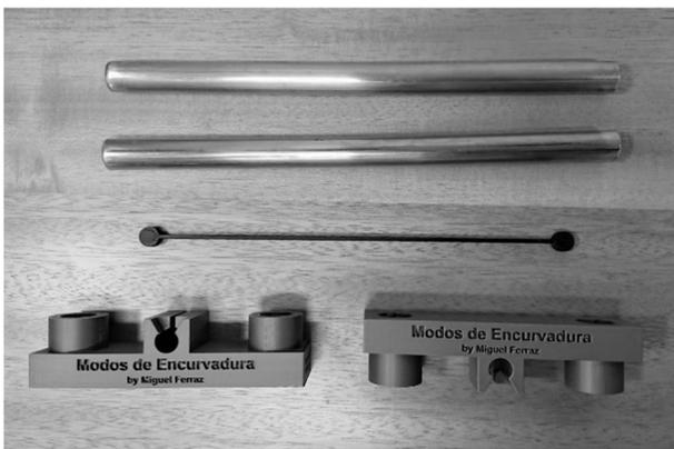
Fig. 7. Finished buckling model parts
