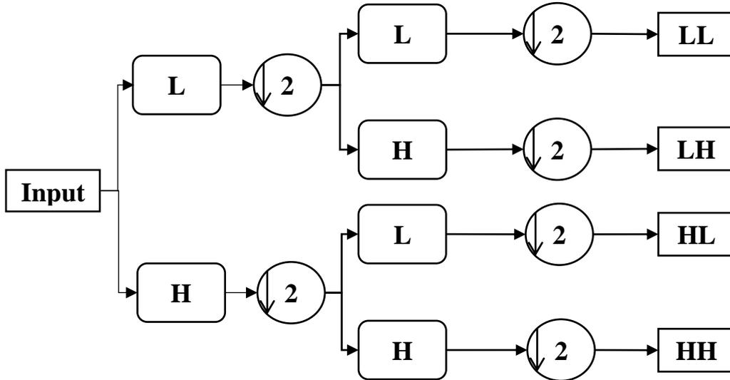
Fig. 4. Example of a one level wavelet signal decomposition.
