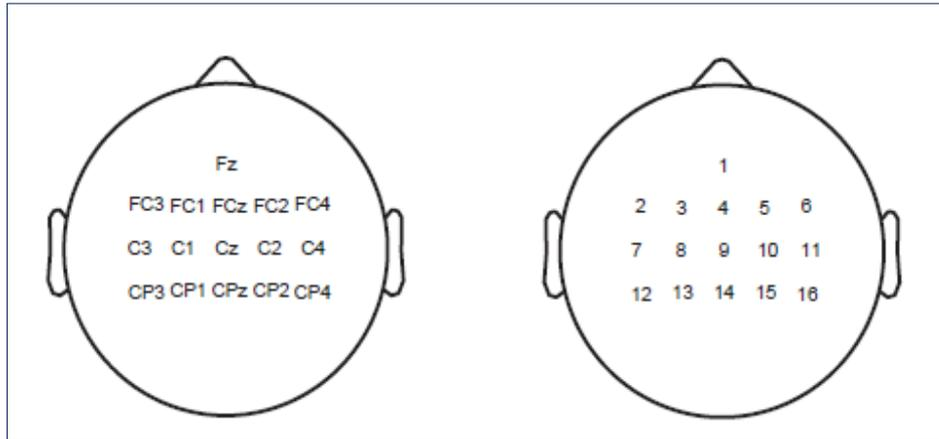
Fig. 5 Layout of the used 16 EEG channels cap.
