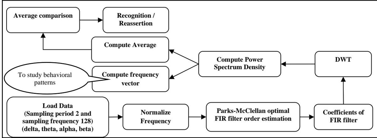
Fig. 2 Detailed methodology for brain EEG signal processing and analysis.
