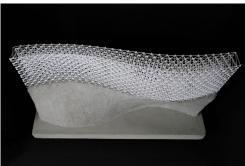
Indirect intervention / reinforcement / formative and additive. To overcome the complex and manual labour process of creating steel reinforcement cages, the "Tailorcrete" research project has explored the automation of this process through the formative process of robotic bending[4].
