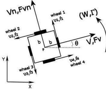
Fig. 2. Geometric parameters and coordinate frames.
