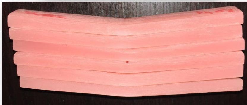
Figure 14. Action of compressive load in the flexural strength test
