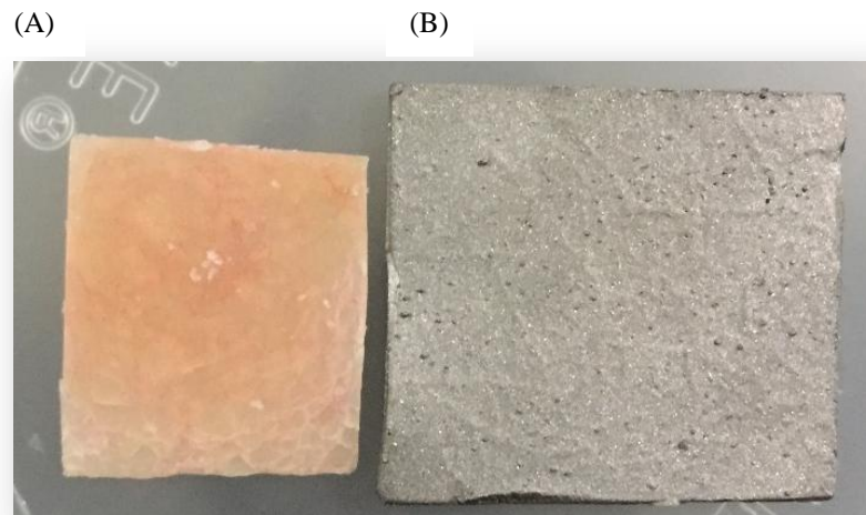
Figure 8. A sample of polymethylmethacrylate resin acrylic (A) and cobalt-chromium alloy (B) coats with a monolayer of graphene.
