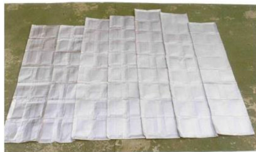
Fig. 2. Thermal blankets made out of old liquid food cartons [7].
