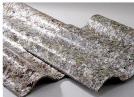
Fig. 3. Roof tile produced with old liquid food cartons [8].
