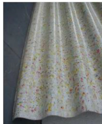
Fig. 4. Eco-tile produced with toothpaste tubes [9].
