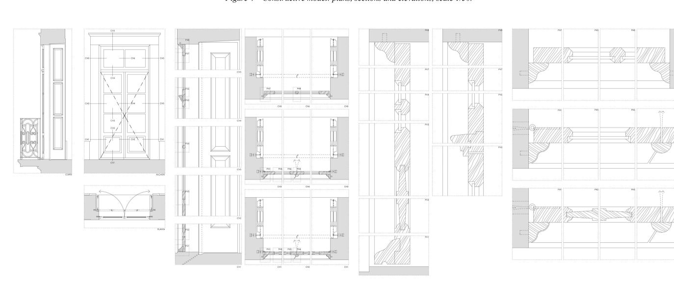
Figure 6 – Example of a balcony window in various scales of detail.
