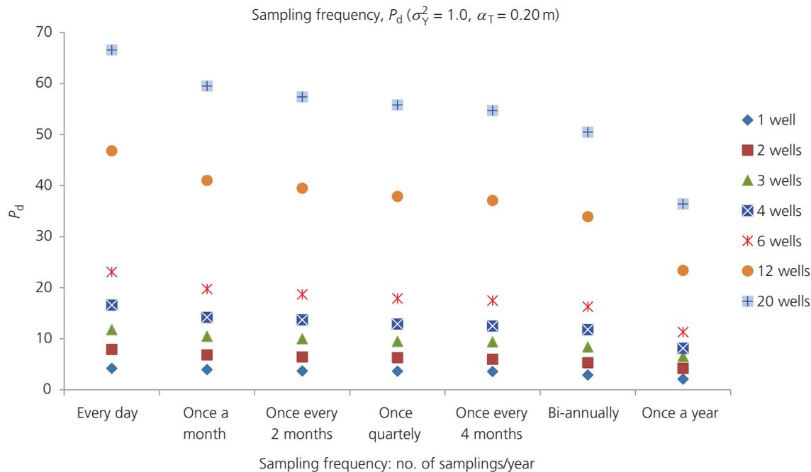
**Figure 6.** Probability of detection,  $P_d$ , plotted against the frequency of sampling for a mild heterogeneous medium (variance of  $\ln K$  is equal to 1, where  $K$  is the hydraulic conductivity and transverse dispersivity,  $\alpha_T$ , is equal to 0.2 m) for several configurations of monitoring wells (Papapetridis and Paleologos, 2011b)
