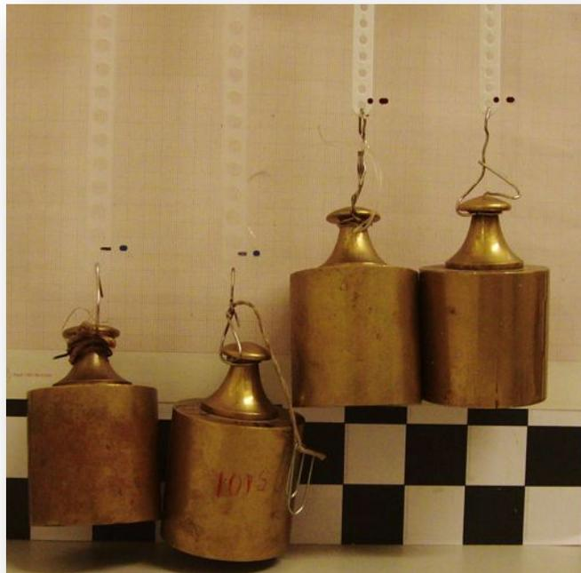
Fig. 8 – View of specimens C5, C6, O5 and O6 with 9,8N calibrated masses in suspension.
