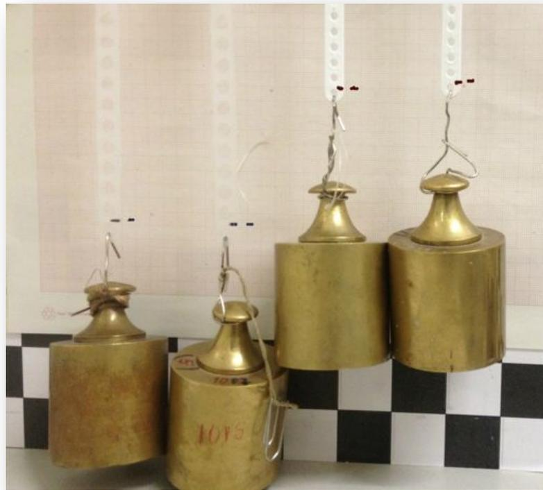
Fig. 9 – Photograph after 18 days (432hours) of constant load tension application. No change in the initial position of the marks occurred.
