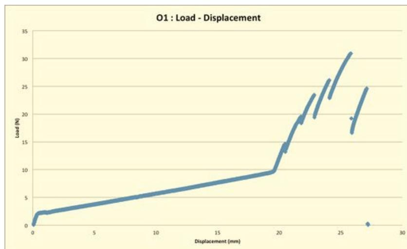
Graph 1 – Tensile test – specimen O1.
