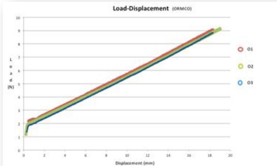
Graph 5 – Linear region of the load-displacement graphs of group O's force modules.
