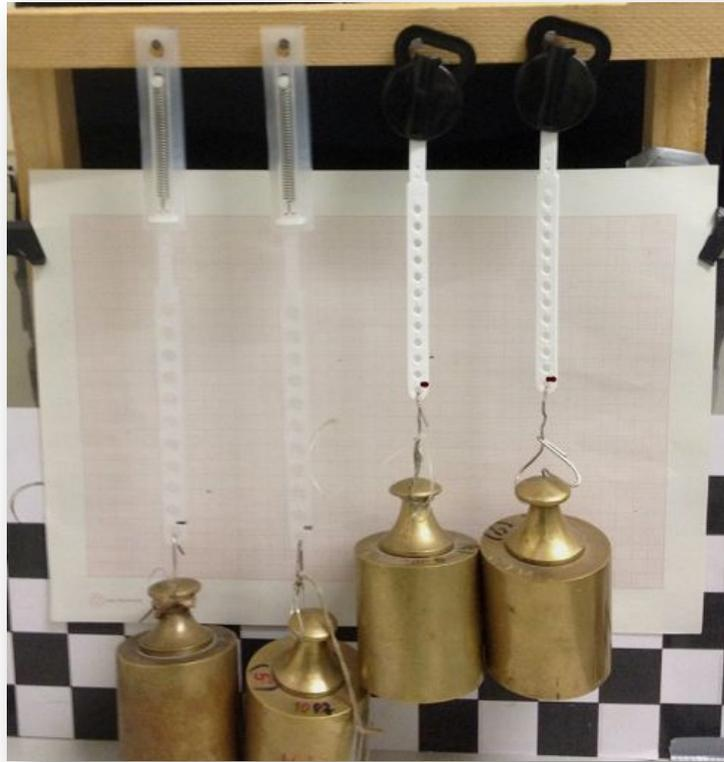
Fig. 7 – Customized support structure for the constant load tension test.
