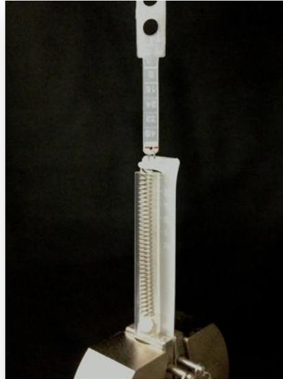
Fig. 5 – Specimen from Ceosa® during tensile test; view of the disengagement of the coil spring from the plastic strap.
