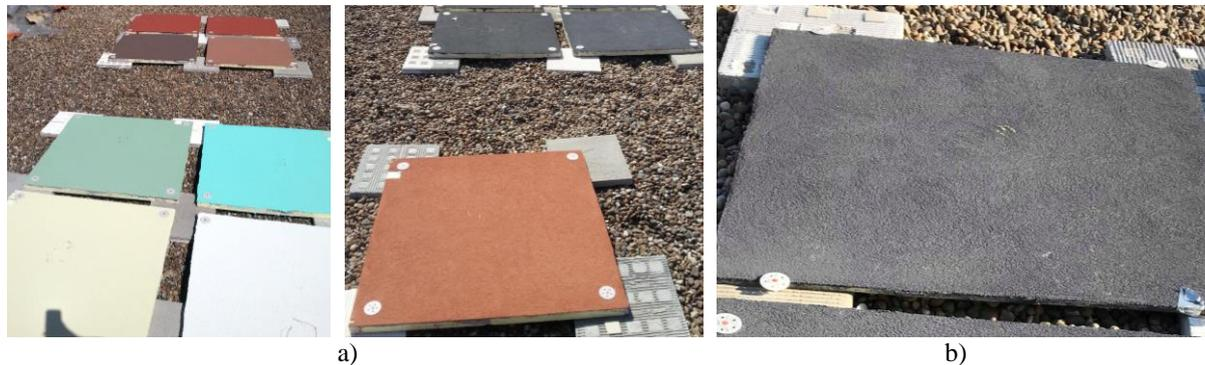
Figure 1: Analysed specimens: a) With insulation layer (EPS); b) Without insulation layer (concrete slab)
