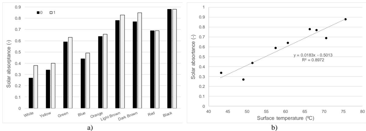
Figure 2: a) Solar absorbance variation; b) Solar absorbance as a function of surface temperature (year 0).
