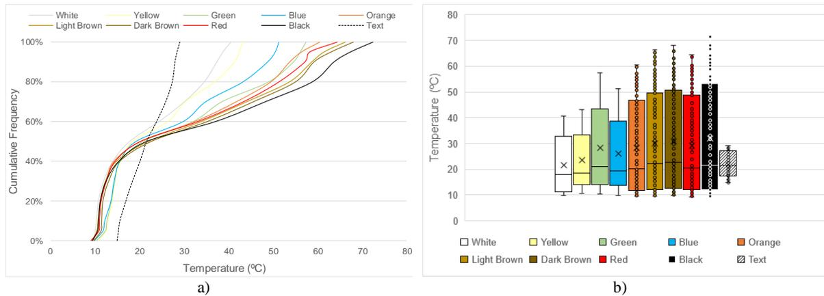
Figure 3: Surface temperature (day of maximum air temperature): a) Cumulative frequencies; b) Box-plots.
