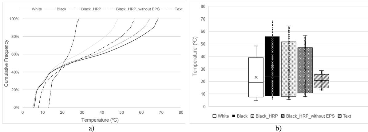
Figure 7: Surface temperature variation (day of maximum air temperature): a) Cumulative frequencies; b) Box-plots.
