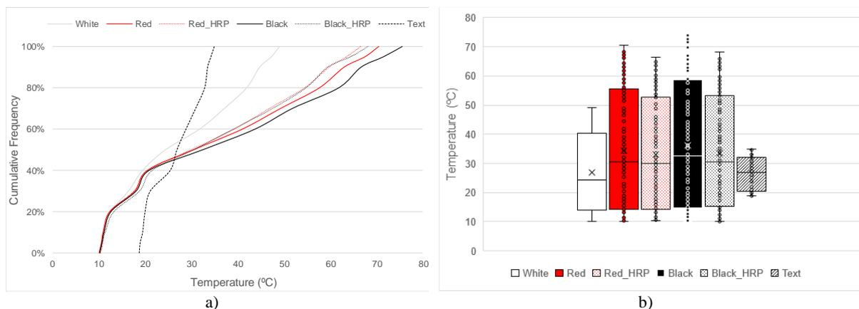
Figure 6: Surface temperature variation (day of maximum air temperature): a) Cumulative frequencies; b) Box-plots.
